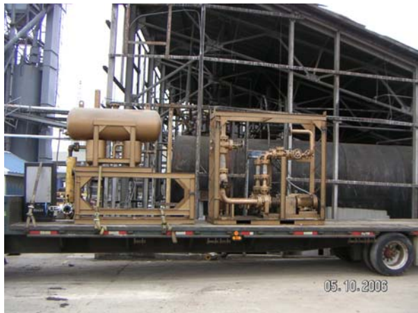
Thermal fluid heater equipment
